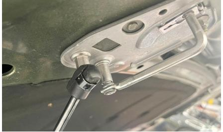
**Step 6** Remove the stock hood prop by rotating it all the way to the right.
