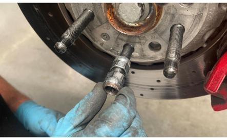
**Step 8** Using a 19mm wrench, tighten the whole assembly from the outermost lug nut.
