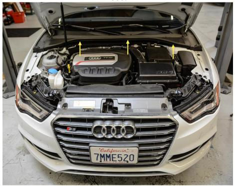
**Step 2**Remove the rubber weather stripping from the cowl cover.
