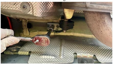
**Step 3**Let the exhaust rest on the driveshaft tunnel brace.
