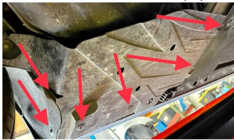
Use a T27 Torx to remove the screws near the side valances.
