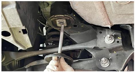
**Step 5**Grease the "rear" inserts for installation.
