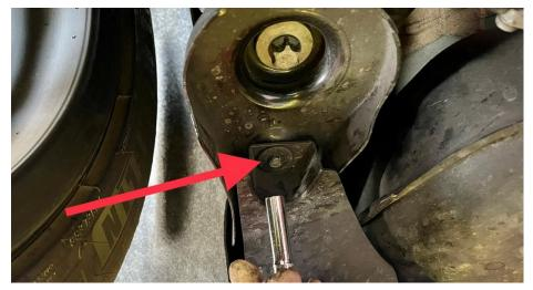
For the remaining push-pins, remove with a flathead.
