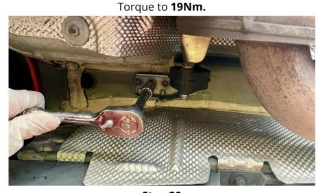
**Step 20**Reattach the underbody trays from step 11.
