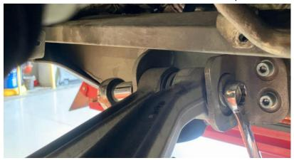
\*The small box mounted to the passenger side of subframe will need to be unlatched. Let it hang while removing the bolt from the subframe mount.
