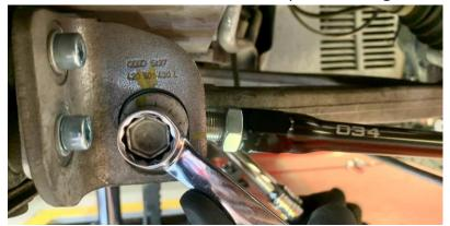
\*Do not torque the bolts down until an alignment has been performed.
