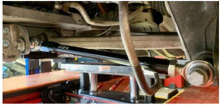
\*We recommend installing with the hexagonal end in the subframe mount to make adjustments much easier.
