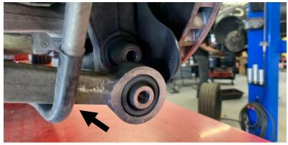
\*Be careful of the emergency brake line when removing the bolt and arm from the car.
