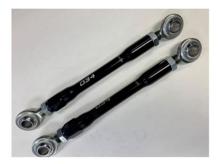
You are now ready to start the installation process. Use the length of the stock component as a starting point for the length of the 034 adjustable end links; expand or compress as best fits your needs
