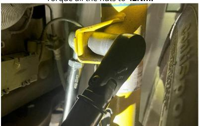
\*If you did not use pole jacks to simulate static ride-height, drop the car down to torque the hardware.
