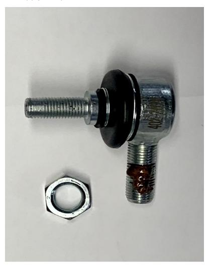
Run the jam nut down the shaft to disperse the anti-seize along the entire threaded portion
