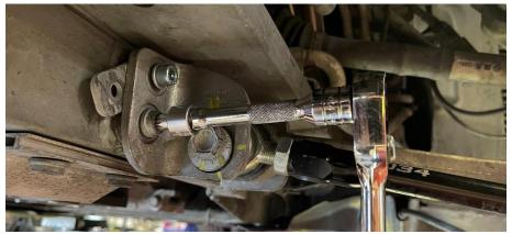
With 6mm Allen, lightly snug the new hardware. The supplied bolts are good for 1-2 shims, so you will need to source longer hardware if using more than 2 shims.
