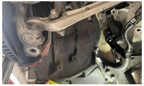
**Step 10** Using a 10mm socket, remove the nut from the ride height sensor, and set the sensor aside.
