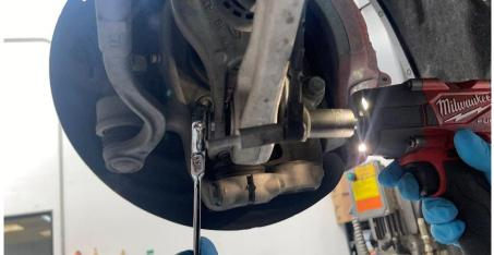
**Step 12** Using a 21mm wrench, remove the nut from the "front" ball joint.
