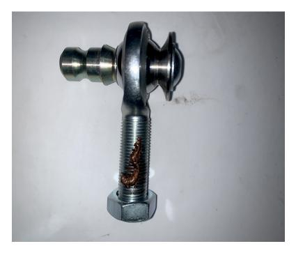
• Leave about 8 threads exposed from the 'bottom' of the shaft
