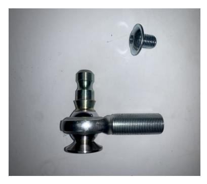
• Apply half packet of anti-seize to spherical heim joint.
