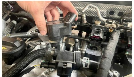
**Step 9** Install the 034 ignition coils.
