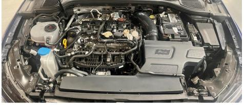
**Step 2** If present, remove the engine cover. **Step 3**
