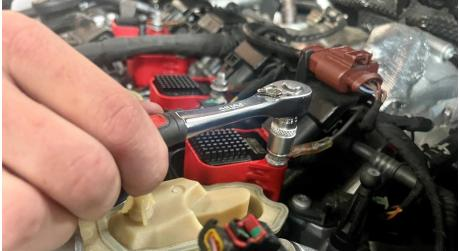
**Step 13** Reinstall the PCV pressure sensor.
