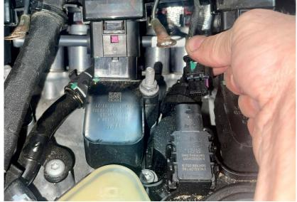
**Step 7** Using a 10mm socket, remove the stud securing the coils to the valve cover.
