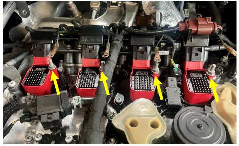
**Step 11** Install the coil harness connectors to the coils.
