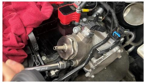
**Step 11** Using a 17mm wrench, tighten the nut on the hardline fitting.
