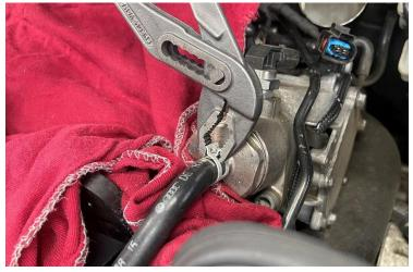
**Step 13** Reinstall the fuel pump sensor.
