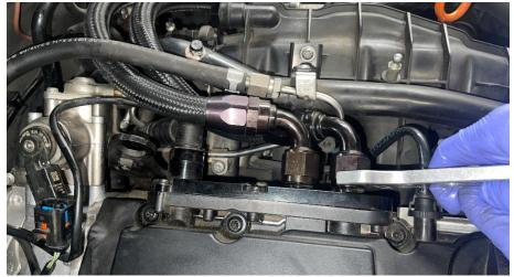
**Step 8** Squeeze and pinch to remove the clips from the fuel pressure sensor and HPFP.
