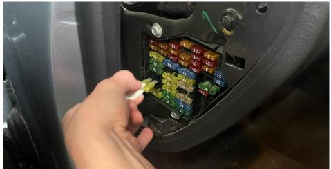
**Step 3** To relieve the pressure, run the car until it dies.
