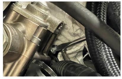
**Step 12** Unscrew the cap from the HPFP bleed screw. Use a 13mm wrench to remove the bleed screw.
