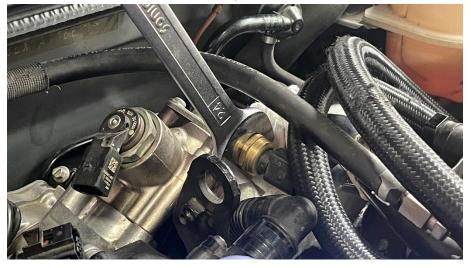
**Step 10** Use a 17mm wrench to remove the high pressure feed line fitting (it's a tight fit).
