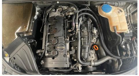
**Step 6** To free up some work space, disconnect the hose and remove the bracket with a 10mm socket.
