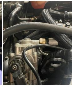
**Step 32** Reinstall/tighten catch can lines.
