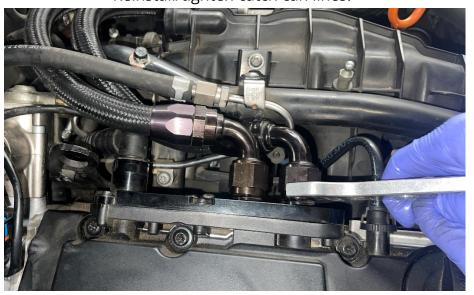
**Step 33** Use a 10mm socket to reinstall bracket.
