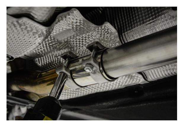
**Step 13 –** Once the rear is secure, tighten the front exhaust clamp completely.
