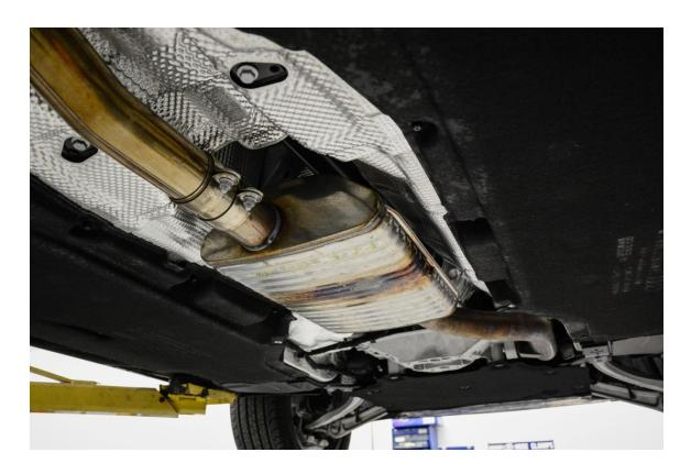
**Step 2** – Align the rear of the 034Motorsport Res-X Resonator Delete with the factory exhaust clamp behind the resonator, and mark the factory exhaust where the front of the 034Motorsport Res-X Resonator Delete terminates.
