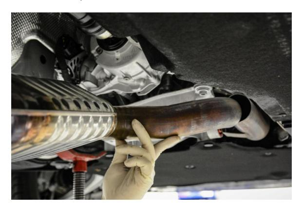
**Step 10** – Slide one of the supplied exhaust clamps loosely over the downpipe. Slide the remaining exhaust clamp loosely over the rear section of the 034Motorsport Res-X Resonator Delete.
