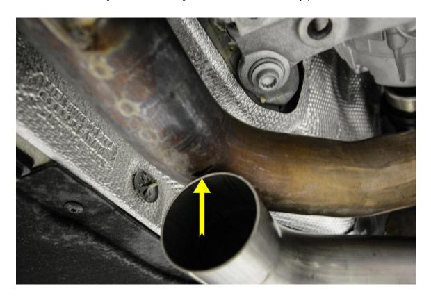
**Step 4** – Support the factory resonator with a jack to hold it in place while cutting the front section of the exhaust.
