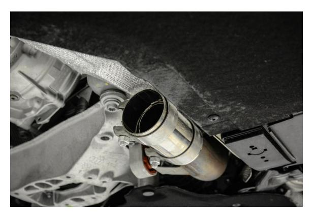
**Step 11** – Lift the 034Motorsport Res-X Resonator Delete into place, slide the clamp so that it is centered on the cut, and gently tighten the front exhaust clamp.
