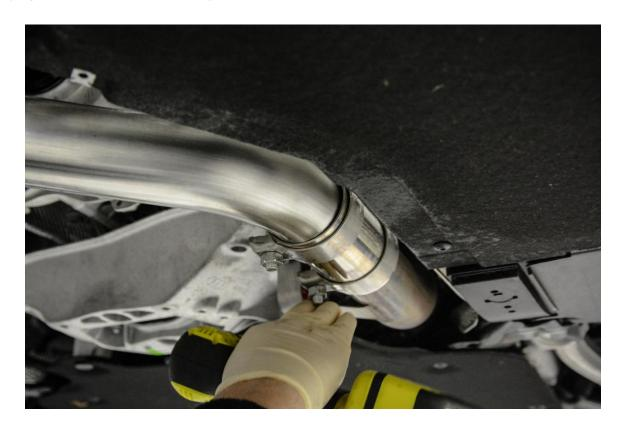
**Step 12 –** Slide the rear exhaust clamp from the 034Motorsport Res-X Resonator Delete halfway over the rear section of the factory exhaust. Ensure the clamp is covering equal amounts of factory exhaust and 034Motorsport Res-X Resonator Delete. Make sure the delete pipe is level with the stock exhaust (i.e. not too high or too low at the elbow). Once aligned, tighten the rear exhaust clamp.
