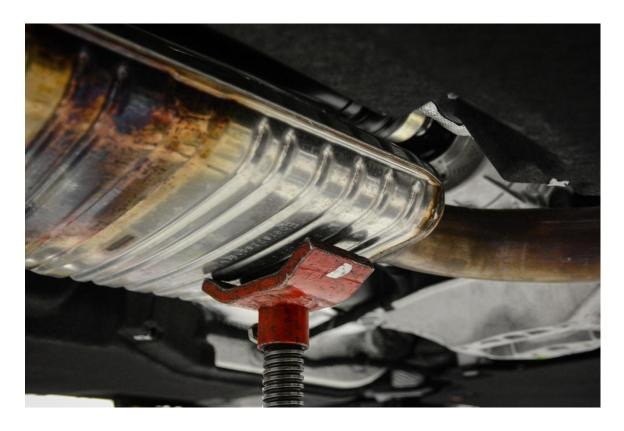
**Step 5** – We found the best way to cut the factory exhaust in front of the resonator was by using a pipe cutter. These can be found at most hardware stores
