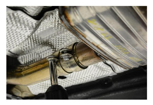
**Step 9** – The resonator should be completely free from the factory exhaust now. Remove this section from underneath the car and take a deep breath.
