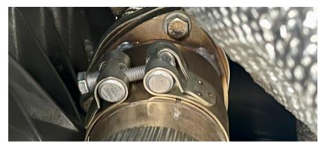
**Step 28** Reinstall the chassis brace.
