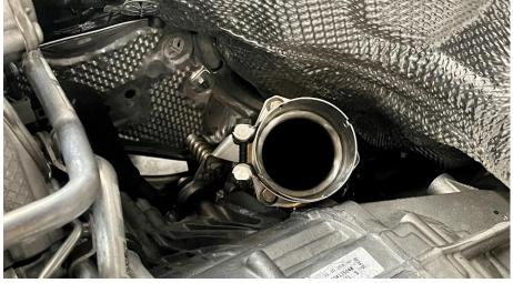
**Step 24** Carefully install the 034 downpipes.
