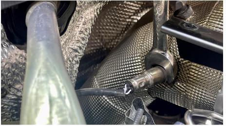
**Step 9** Using a T30 Torx bit, loosen the v-band clamps on each downpipe right off of the turbochargers.
