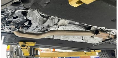
**Step 22** Using a 10mm triple-square, reinstall the exhaust dampeners. Leave loose for adjustments.
