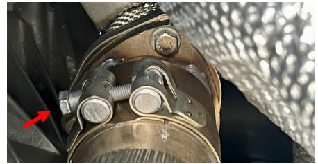
**Step 11** Carefully remove the downpipes from the engine bay. This may require using some lubricating spray and lots of wiggling/twisting.
