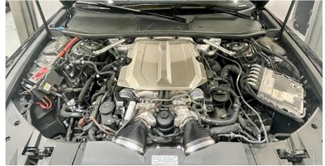
Step 3 Using a T30 Torx bit, remove the heat shield covering the turbochargers.
