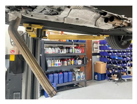
\*We could easily not get the passenger side assembly out without damaging the lower heat shielding near the front subframe. Instead, we pushed it up and forward, into the engine bay, to better access the flange hardware from inside the engine bay.
