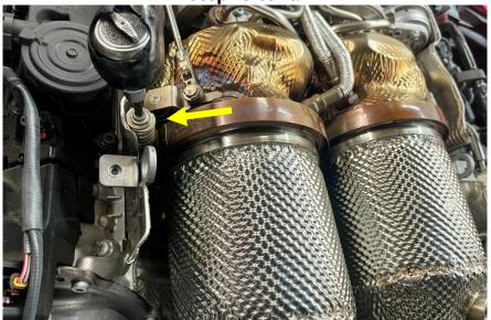
**Step 26** Using a 22mm wrench, reinstall the oxygen sensors. (Tool not shown.)
