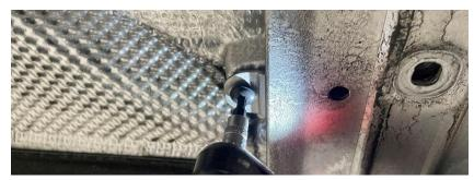
Step 18 Using a 15mm socket, loosen the exhaust clamps connecting the midpipes to the rear exhaust pipes.
