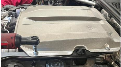
**Step 34** Reinstall the engine cover.
