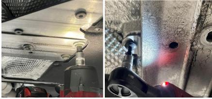
**Step 29** Reinstall the lower heat shields near the subframe.
