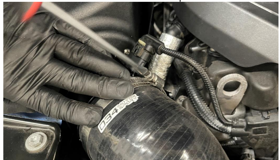
Step 21 Reconnect the intake hose to the MAF housing and secure it with the hose clamp.
