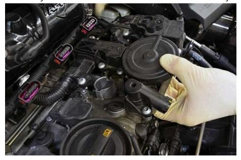
\*Be careful to avoid dropping any screws into the holes in the valve cover.
